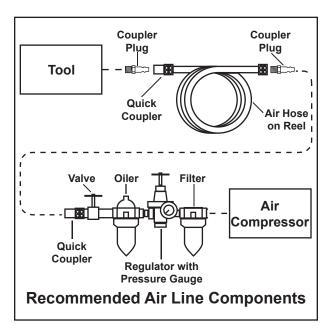
NOTE: For best service, you should incorporate an oiler, regulator, and in-line filter as shown above. Hoses, couplers, oilers, regulators and filters are all available at Harbor Freight Tools.
